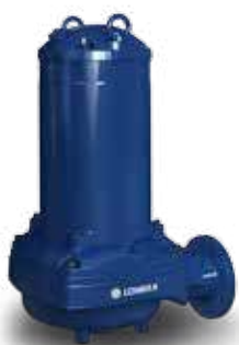
Lowara 1330 Non-clog Maximum flow 310 l/s Maximum pressure 74 m Motor Rating 10 - 24 kW Outlet 100 - 250 mm Weight 300 - 420 kg
