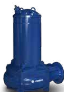
Lowara 1335 Non-clog Maximum flow 492 l/s Maximum pressure 55 m Motor Rating 18 - 50 kW Outlet 150 - 300 mm Weight 580 - 760 kg
